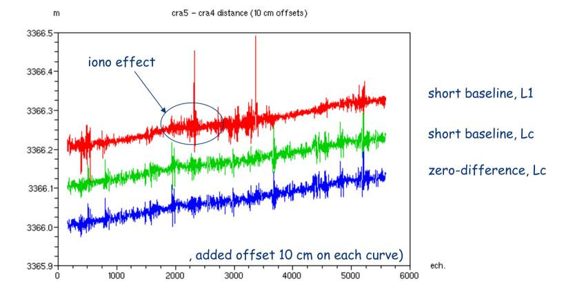
Absolute positioning allows same performance as the short baseline solution (dual frequency)
